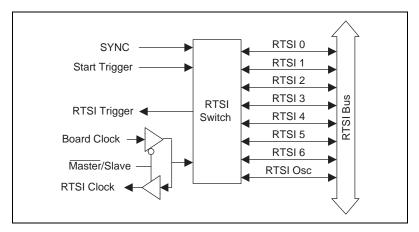
Figure 2-14. RTSI Trigger Lines and Routing for the NI 5401 for PCI
